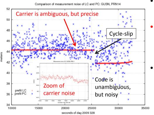
Note: Figure shows the noise of **code** and **carrier** prefitresiduals, which are the <u>input data for navigation equations</u>.
