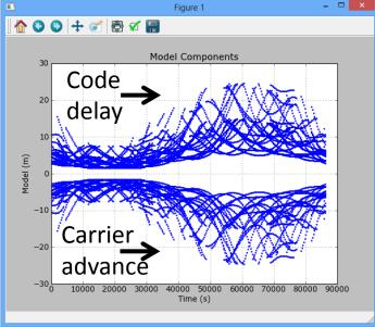
Ionosphere delays code and advances carrier measurements.
