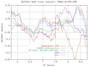
Figure 5: Example of the improvement in the  $\Delta \nabla$  STEC interpolation for the rover receiver, when a real-time tomographic ionospheric model –constrained with the  $\Delta \nabla$  STEC in the reference receivers– is used instead of a linear interpolation model (using the reference stations UCLU, WILL and GWEN in the North-America network). In this dataset the ionosphere presents small scale ionospheric disturbances.
