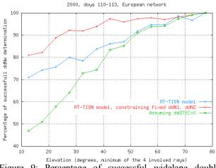
Figure 9: Percentage of successful widelane double integer ambiguity determination as a function of the elevation –of the lowest satellite of the involved rays in each double difference–, for the European network, and in the Solar Cycle maximum peak (222, days 110-113).
