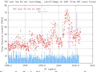
Figure 8: Total Electron Content over Europe (longitude=10 deg., latitude=47.5 deg.), obtained from the UPC ionex files –computed in the framework of the IGS ionospheric project–. The beginning of the data analyzed in scenario 2 and scenario 3 are indicated with vertical arrows (days 110 and 194 of year 2000). The Kp index is also represented.
