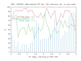
Figure 12: Percentage of successful widelane double integer ambiguity determination as a function of time, for the European network, during several consecutive large geomagnetic storms in the Solar Cycle max. (2000, 110-113). The results neglecting  $\Delta \nabla$  *STEC* are also plotted.
