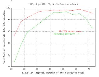
Figure2: Percentage of successful widelane double integer ambiguity determination as a function of the elevation of the lowest satellite, for North-American network (1998, Days 118-120). The results for both tomographic model and neglecting  $\nabla\Delta$ STEC are indicated.
