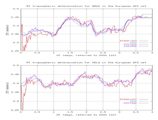
Figure 10: Real-time tropospheric determination using the presented approach (RTROP-OTF), compared with real-time determination also with broadcast orbit relaxation (RTROP), and the corresponding postprocessed determination (TROP), including the IGS one, IGSTROP, and the PPPTROP, all for several reference stations of the European network, in the Solar Maximum peak, days 2000 110-113 (scenario 2).
