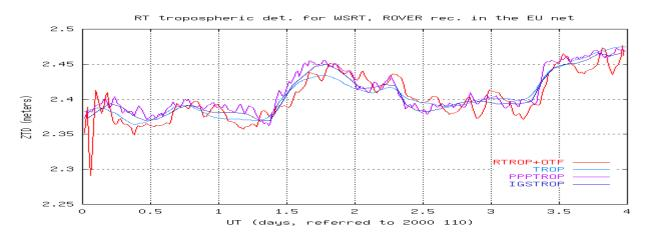
Figure 11: Real-time tropospheric determination of the *rover* receiver WRST, using the presented approach, compared with real-time determination with orbit relaxation, and postprocessed determinations, including the IGS one, also for Scenario 2.
