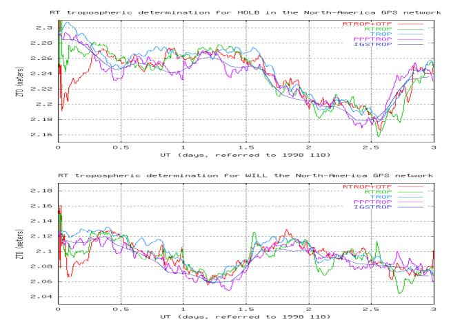
Figure 3: Real-time tropospheric determination using the presented approach (RTROP-OTF), compared with real-time determination also with broadcast orbit relaxation (RTROP), and the corresponding postprocessed determination (TROP), including the IGS one, IGSTROP, and the PPPTROP, all for several reference stations of the Nort-America network.
