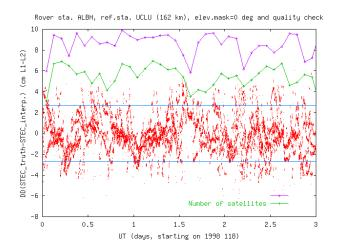
Figure 6: Success in the  $\Delta \nabla$  STEC interpolation to the rover receiver ALBH (points within the limits +/-2.7 cm).
