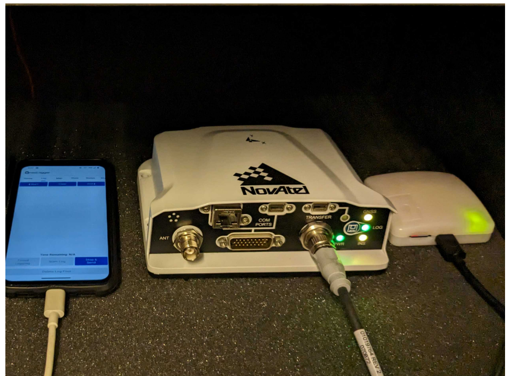
Figure 1. Data collecting experiment setup. From left to right: Samsung Galaxy Note10, NovAtel PwrPak7, Rokubun Argonaut.
